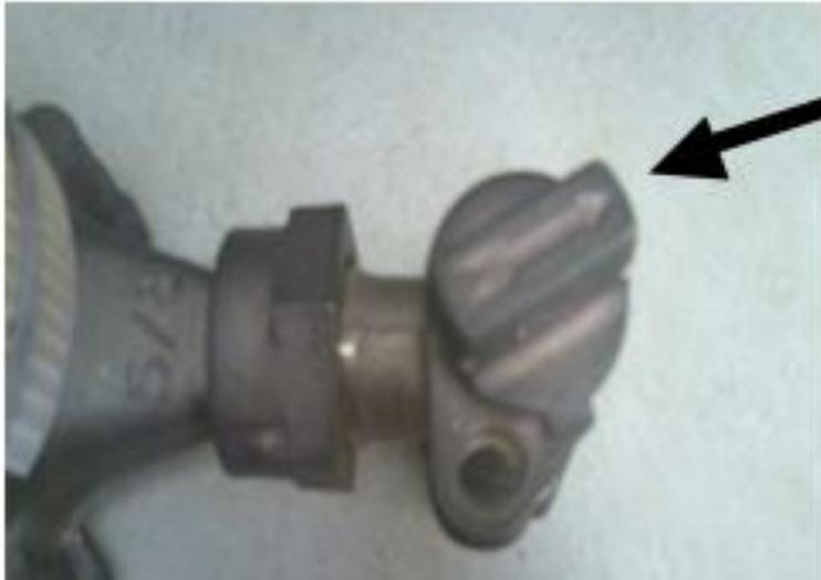
CUT-OFF VALVE IN THE OFF POSITION
