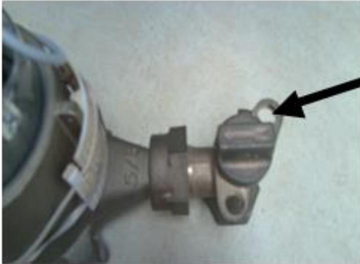
CUT-OFF (VALVE IN THE ON POSITION)
