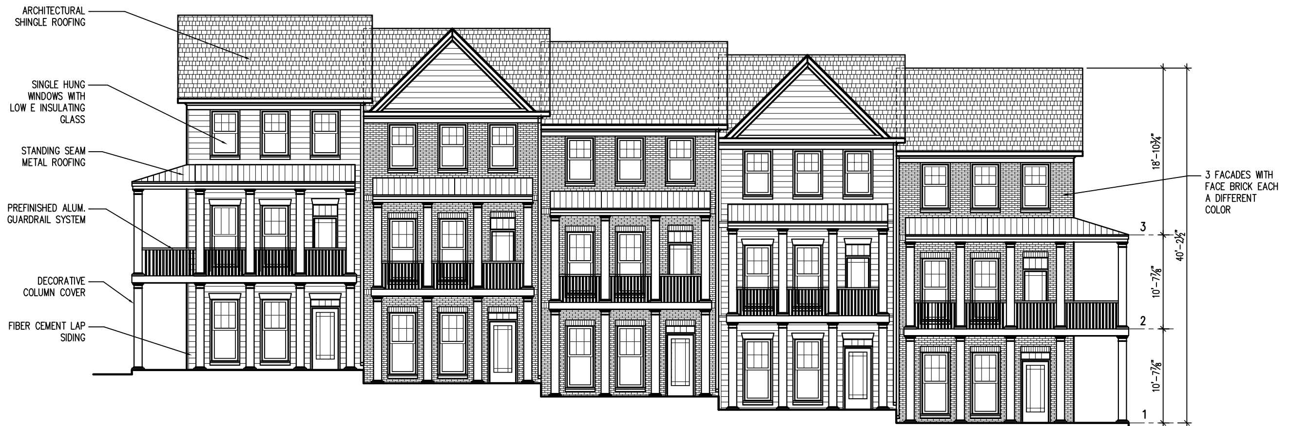
BUILDING T1B - STREET ELEVATION
